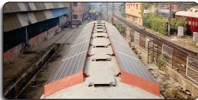
3.6 KWp SPV Power pack installed on train coach
